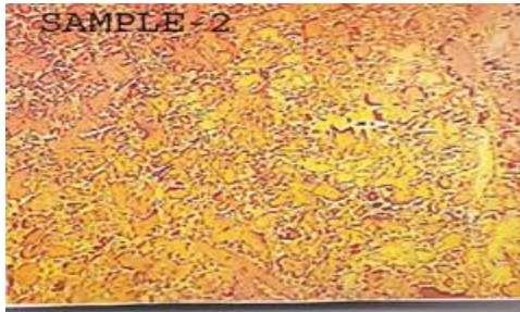
Microstructure of Cu-Al 2 O 3 at 80%- 20%
